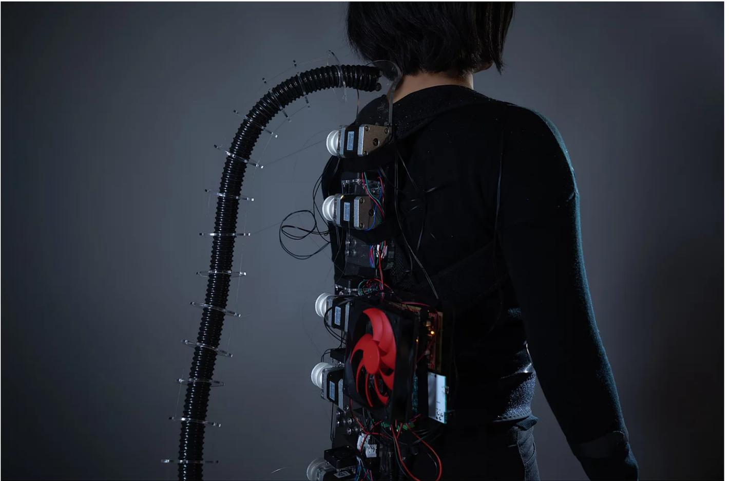
Arduino, stepper motors, LDR sensors
