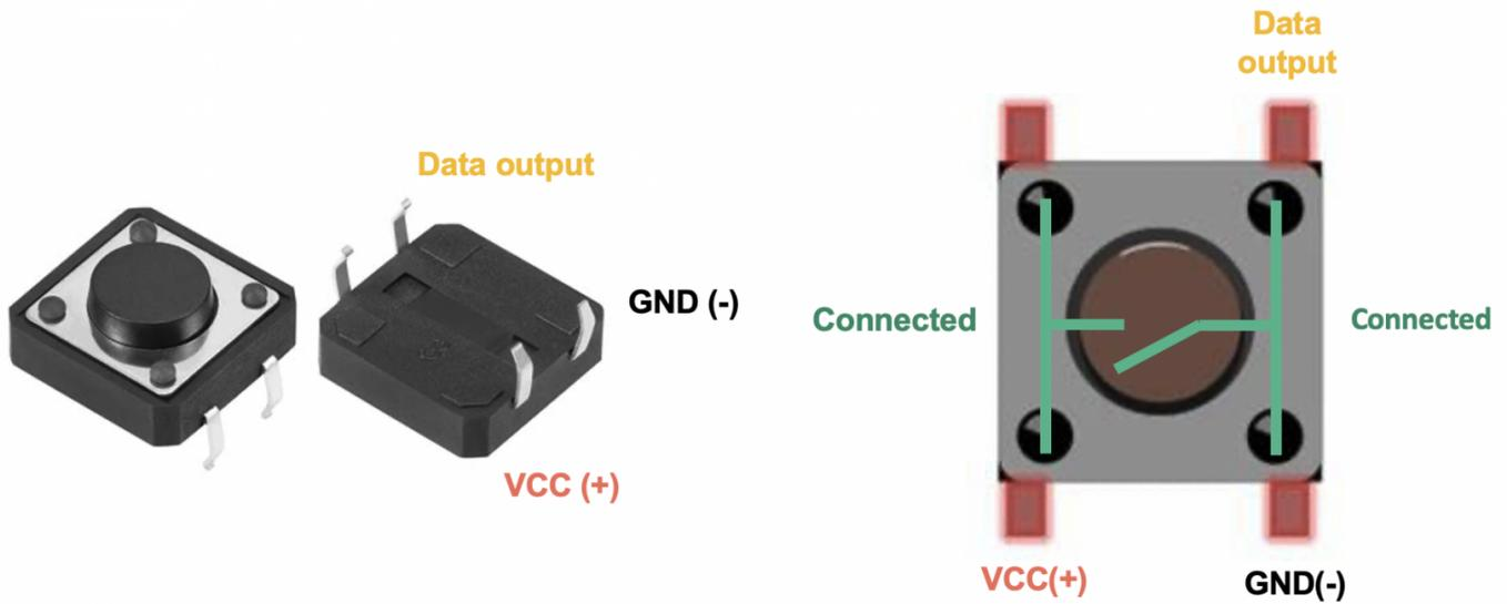
It's not possible however to do this otherwise when you apply 5V by closing the circuit you would create a short circuit, instead we connect the Arduino pin through a high value 10KΩ resistor to ground, this allows the circuit to quickly reach 0V when the button is released but prevents large amounts of current flowing when the button is pressed.
