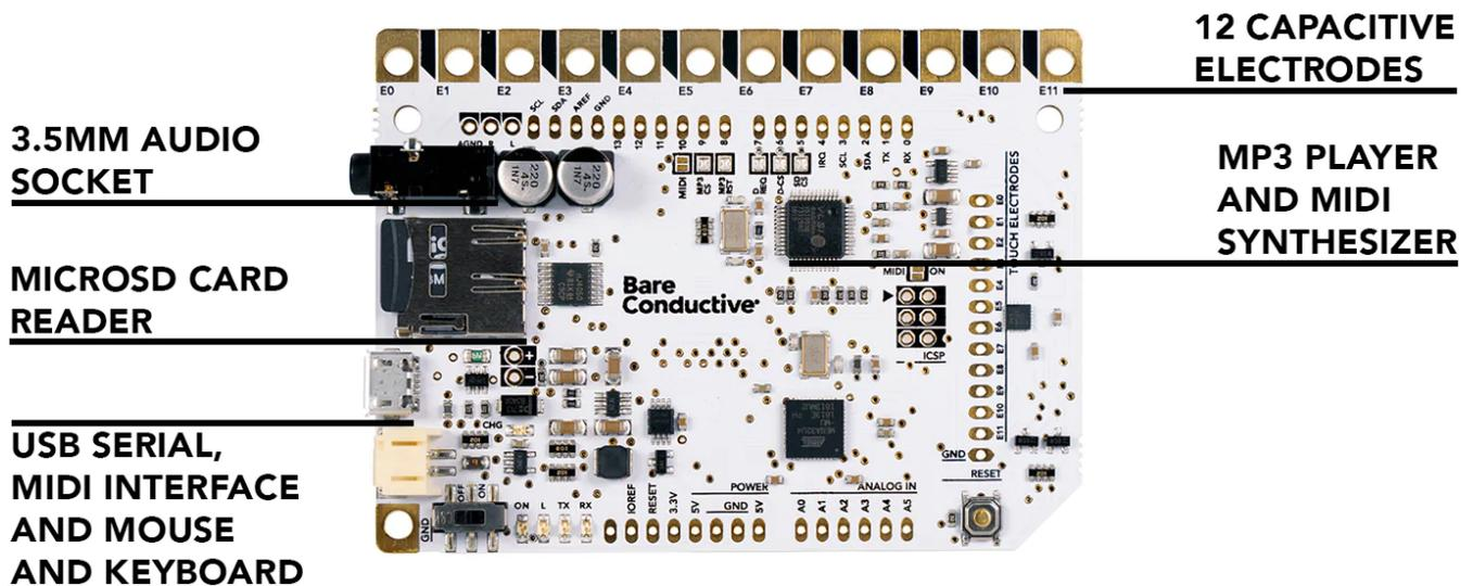
In short, the Touch Board is a pre-built Arduino that combines the functions of **play MP3** and **capacitive touch sensing**, but you can do more than that. If you don't have the Touch Board, you can still do the same things following the above two tutorials.
