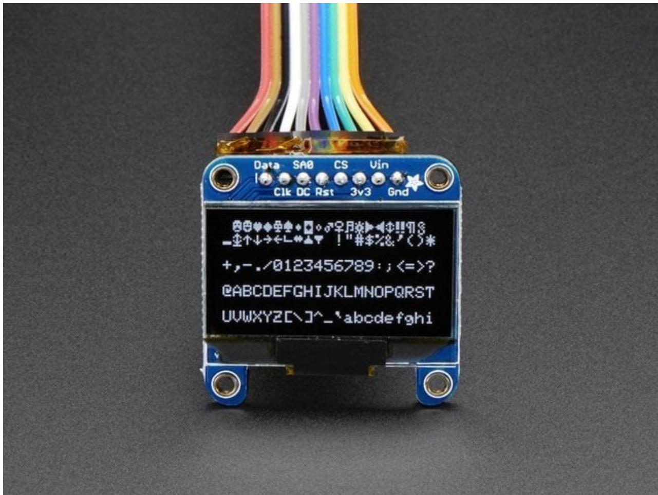
In this tutorial, we will be using Adafruit SSD1306 128 x 64 OLED with I2C communication. It can support SPI communication as well.
